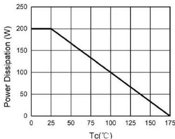
Fig.3 Power Dissipation
