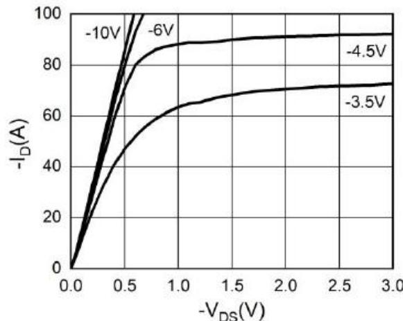
Fig.1 Output Characteristics
