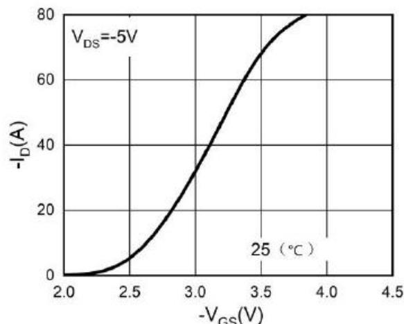
Fig.2 Transfer Characteristics
