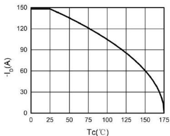
Fig.4 Drain Current
